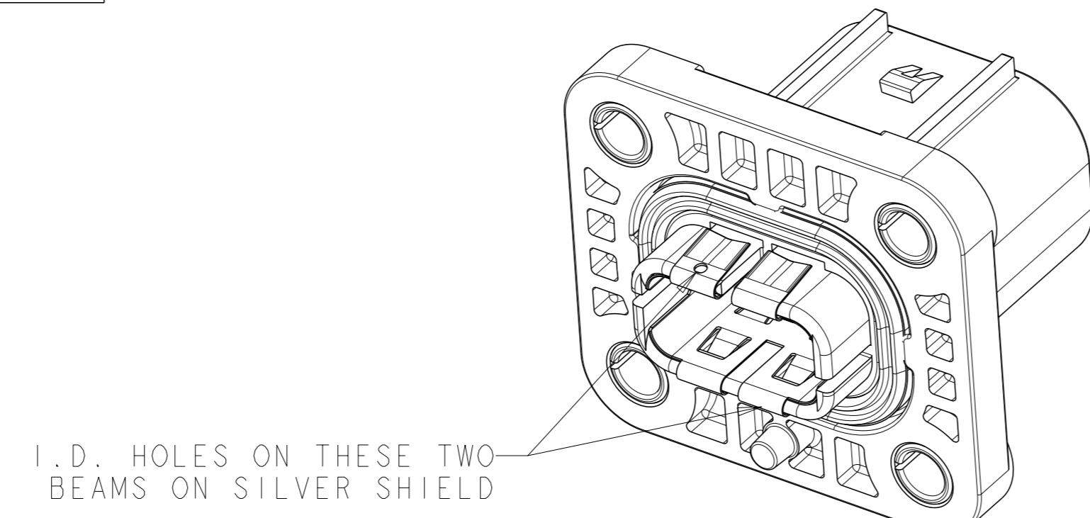
I.D. HOLES ON THESE TWO BEAMS ON SILVER SHIELD
