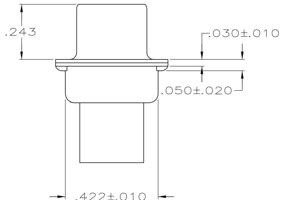
1. CONNECTOR ACCEPTS SIZE 20 DF SOCKET CONTACTS, RETENTION TINES ARE AN INTEGRAL PART OF INSERT.
