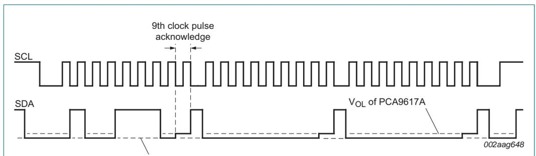
Fig 9. Bus B (2.2 V to 5.5 V) waveform
