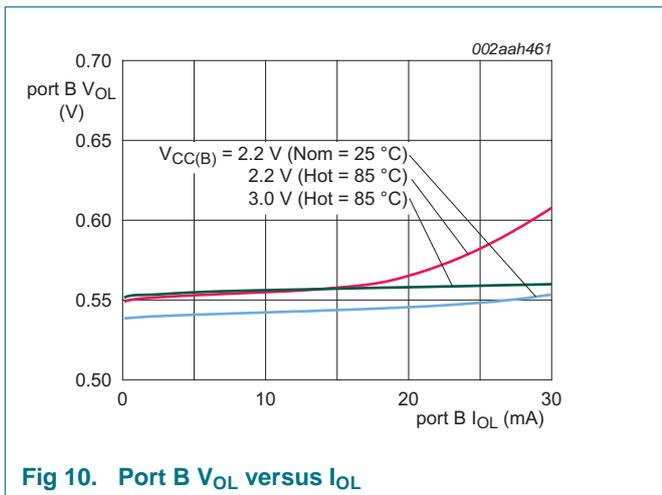
Fig 10. Port B  $V_{OL}$  versus  $I_{OL}$
