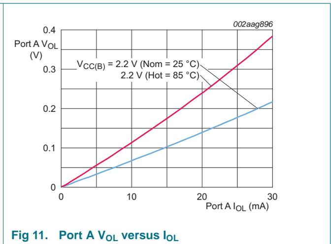
Fig 11. Port A  $V_{OL}$  versus  $I_{OL}$
