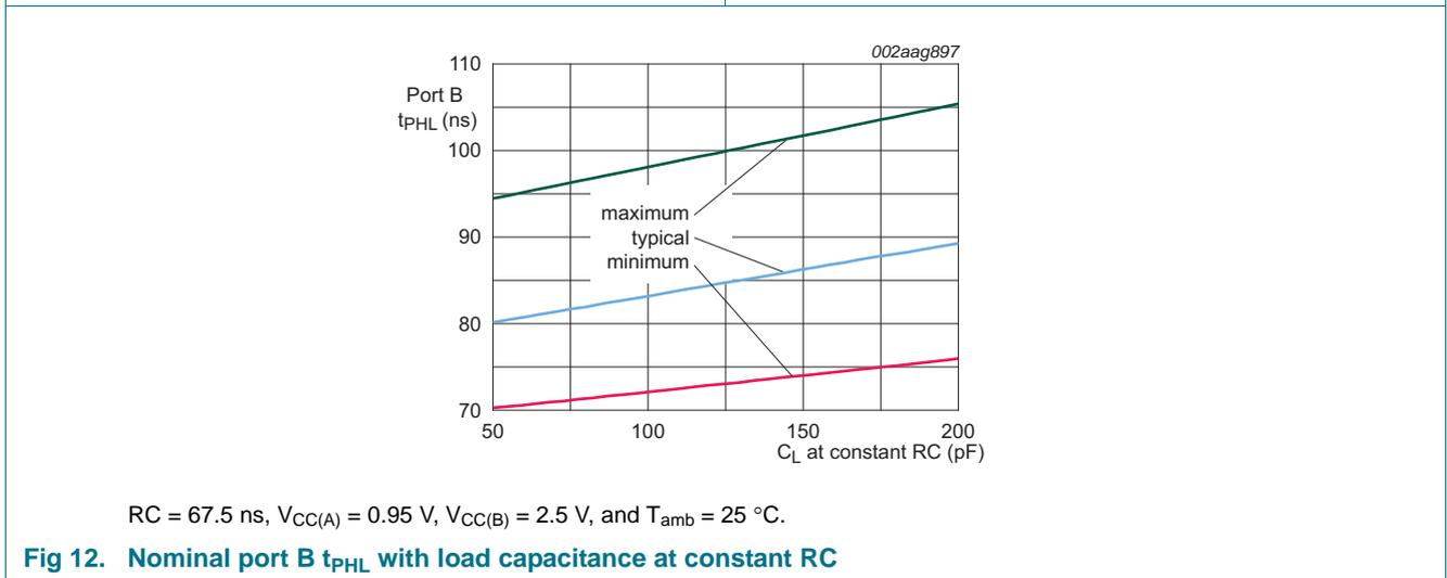
Fig 12. Nominal port B  $t_{PHL}$  with load capacitance at constant RC
