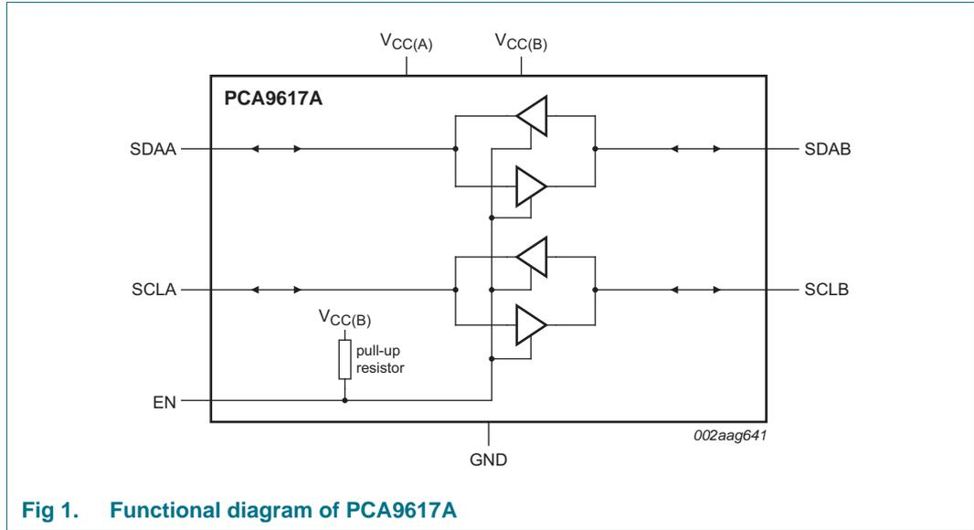
Fig 1. Functional diagram of PCA9617A
