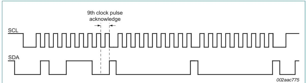
Fig 8. Bus A (0.8 V to 5.5 V bus) waveform
