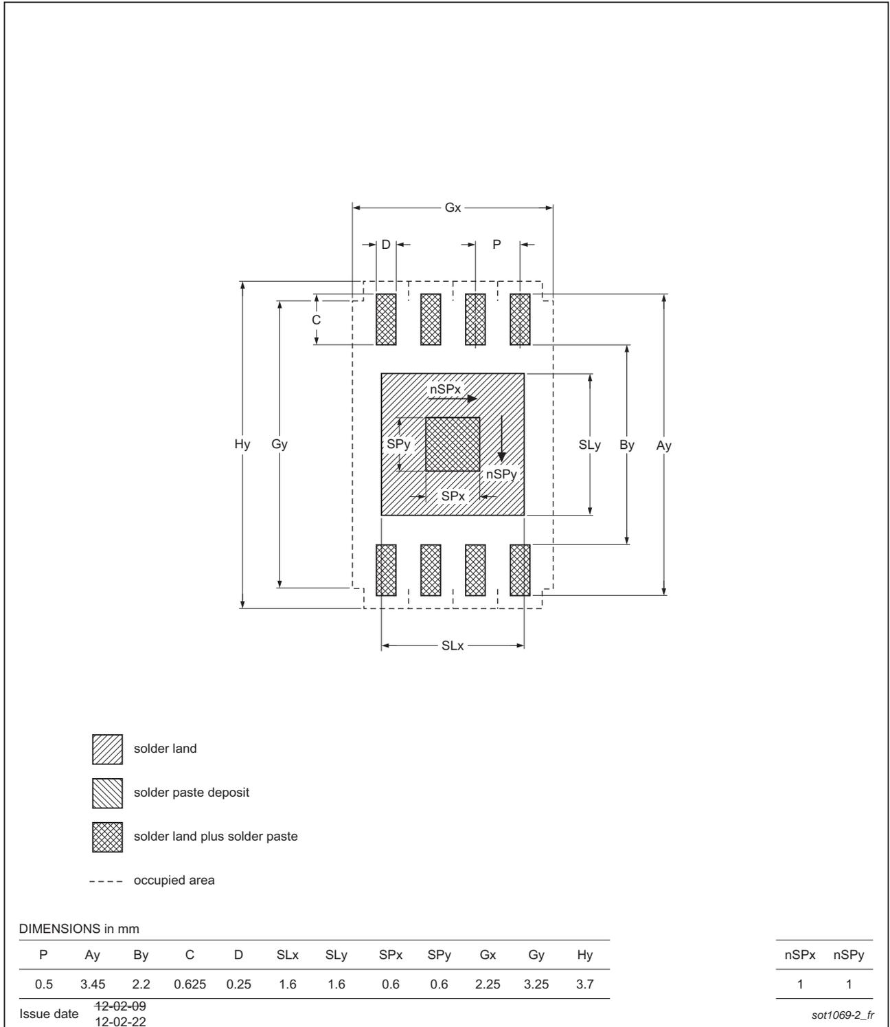
Fig 22. PCB footprint for SOT1069-2 (HWSON8); reflow soldering
