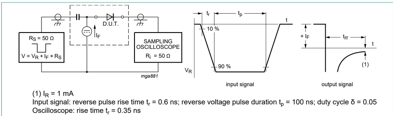
**Fig. 5. Reverse recovery time test circuit and waveforms**
