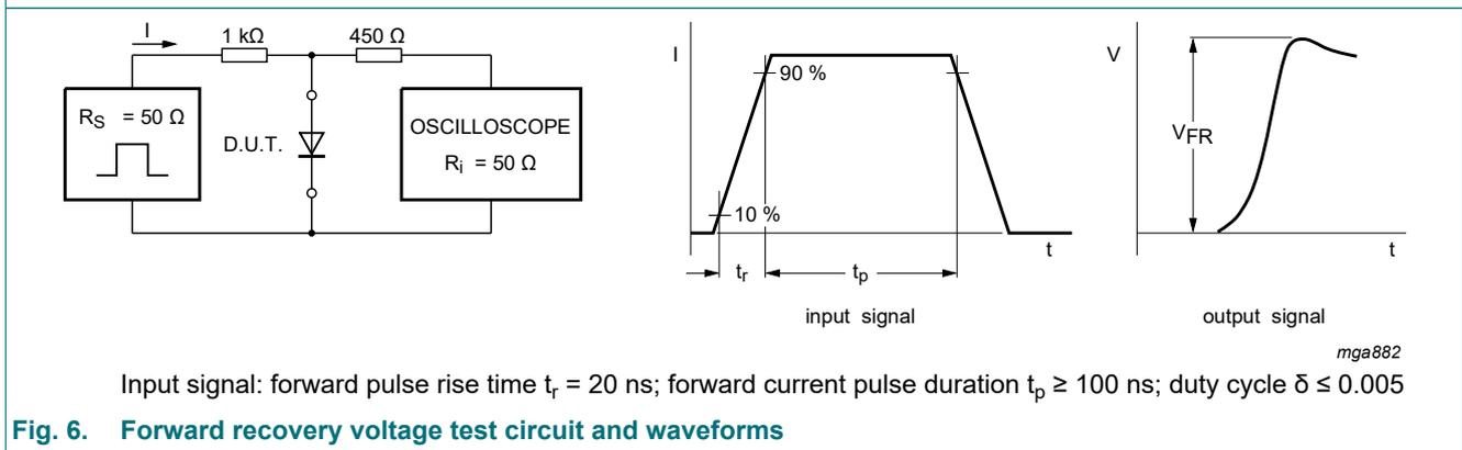
**Fig. 6. Forward recovery voltage test circuit and waveforms**
