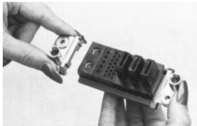
4. Position end caps over locking rail ends and secure using Phillips head screws.
